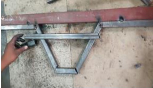
Fig. 5: Fabrication of main frame
